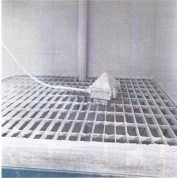
Figure D: DUT after IP 6X Test.
