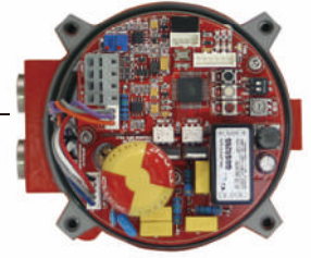
RPC (Option) (Remote Position Controller) Input & Output Signal 4~20mADC
